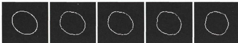
Fig. 3. Gradual failure of the AAS monument tracing technique due to decreasing shape contrast. As edge evidence declines, the extracted shape tends towards a circle. (1) Ideal edge map, (2) result at contrast 21%, (3) result at contrast 18%, (4) result at contrast 12%, (5) result at contrast 9%
