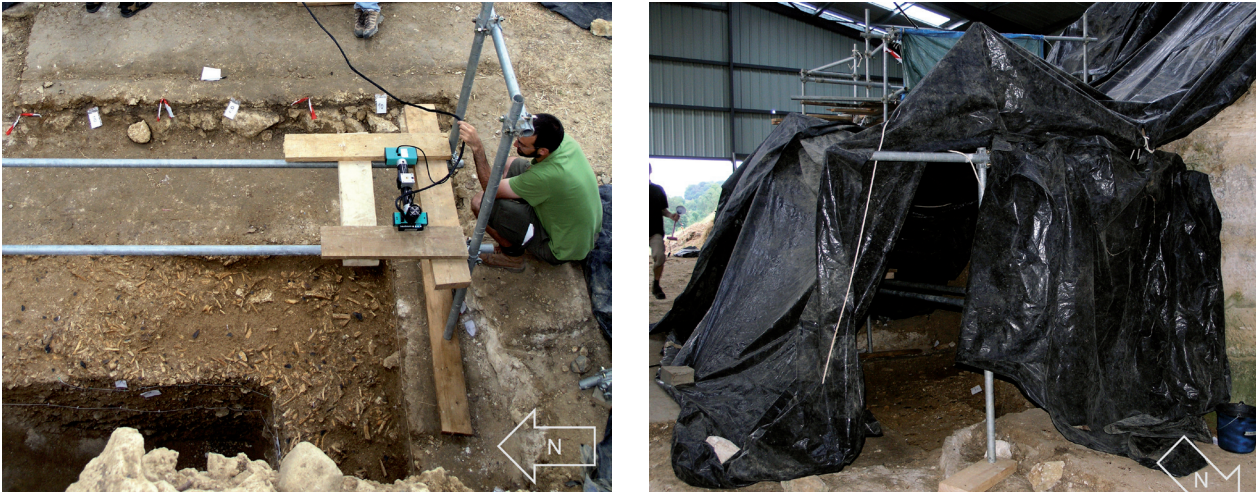
Fig. 2. Frame made from scaffolding tubes with wooden sledge holding the sensor unit of the scanner over the bone-bed (left). The opaque tarp used to block daylight from the bone bed (right) (photos by Steffen Lättsch).
