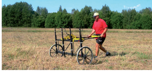
Fig. 5. Magnetometer measurements with a Förster magnetometer system. Four gradiometer probes are mounted with 50 cm horizontal spacing onto the cart. The cart is pushed in zig-zag mode along 50 m long parallel profile lines that are spaced in 2 m intervals on the ground.
