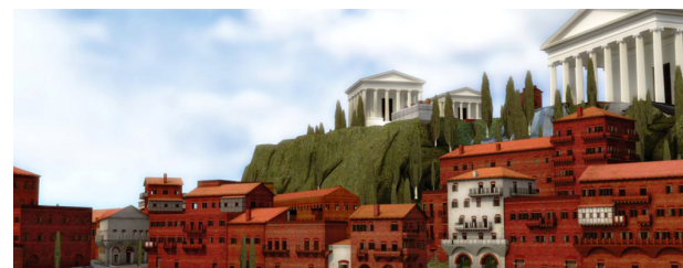
Figure 7. An offline rendered scene with temples. Only a single CGA shape rule set describing Classical architecture was used. The different temple variations emerge by adaptation to the initial shape and/or rule input parameter modifications. The rendering was created using Autodesk Maya and Mental Images' Mental Ray.
