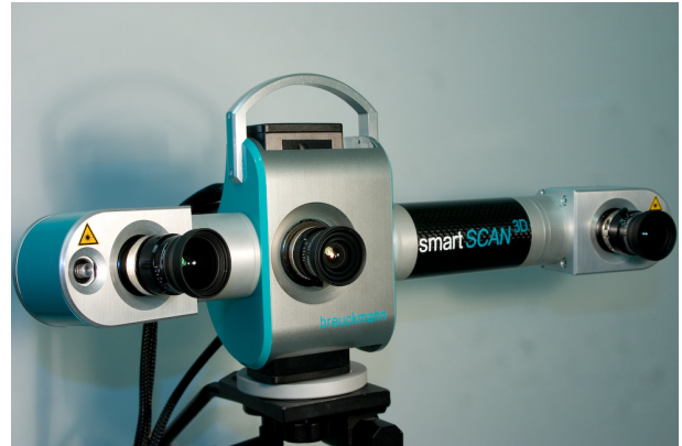
Figure 1. 3D-surface scanner smartSCAN 3D .
