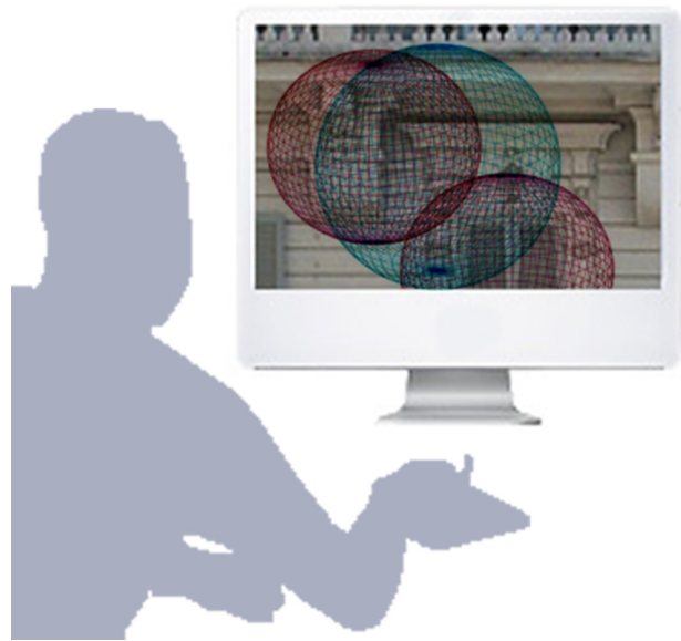
Fig. 3. Interactive 3D Viewer with the viewing zone VZ represented as a "green sphere" and two information zones IZ represented as "red spheres".
