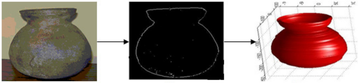
Figure 12a. Input media is digital image acquired through CCD camera, b. extracted edges, c. reconstructed pot.
