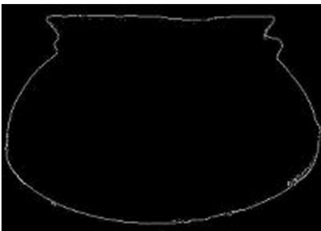
Figure 5b. The extracted edges through the use of the Sobel filter.
