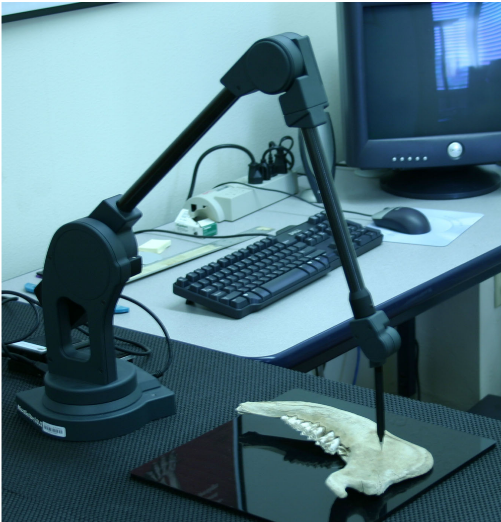
Figure 2. Immersion Microscribe Point Digitizer.
