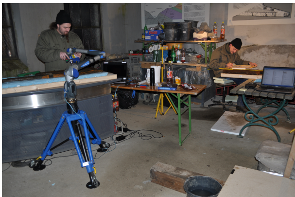
Figure 5: The close range laser scanning (left) and the archaeological drawing (right) of the wooden boards.
