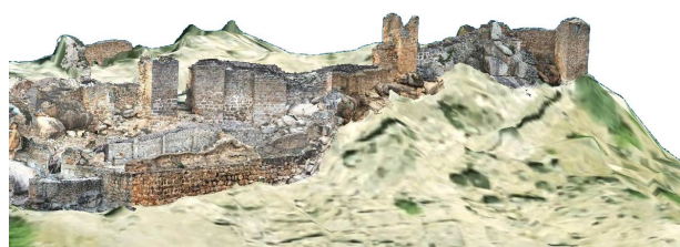
Figure 7: Screenshot of the virtual model supported on the digital terrain model generated by a photogrammetric flight.
