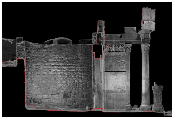
Figure 6: Section through Hadrian's Temple created from point cloud from 3D laser scanning.
