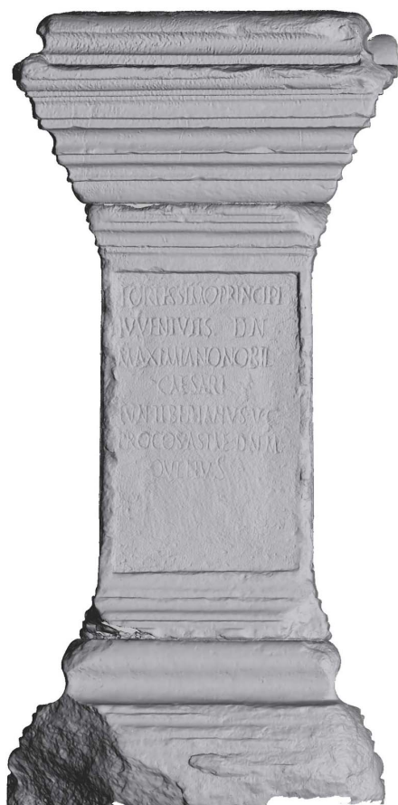
Figure 5: Final result: An inscribed statue base as ortho-projection, compiled from fringe projection scans.
