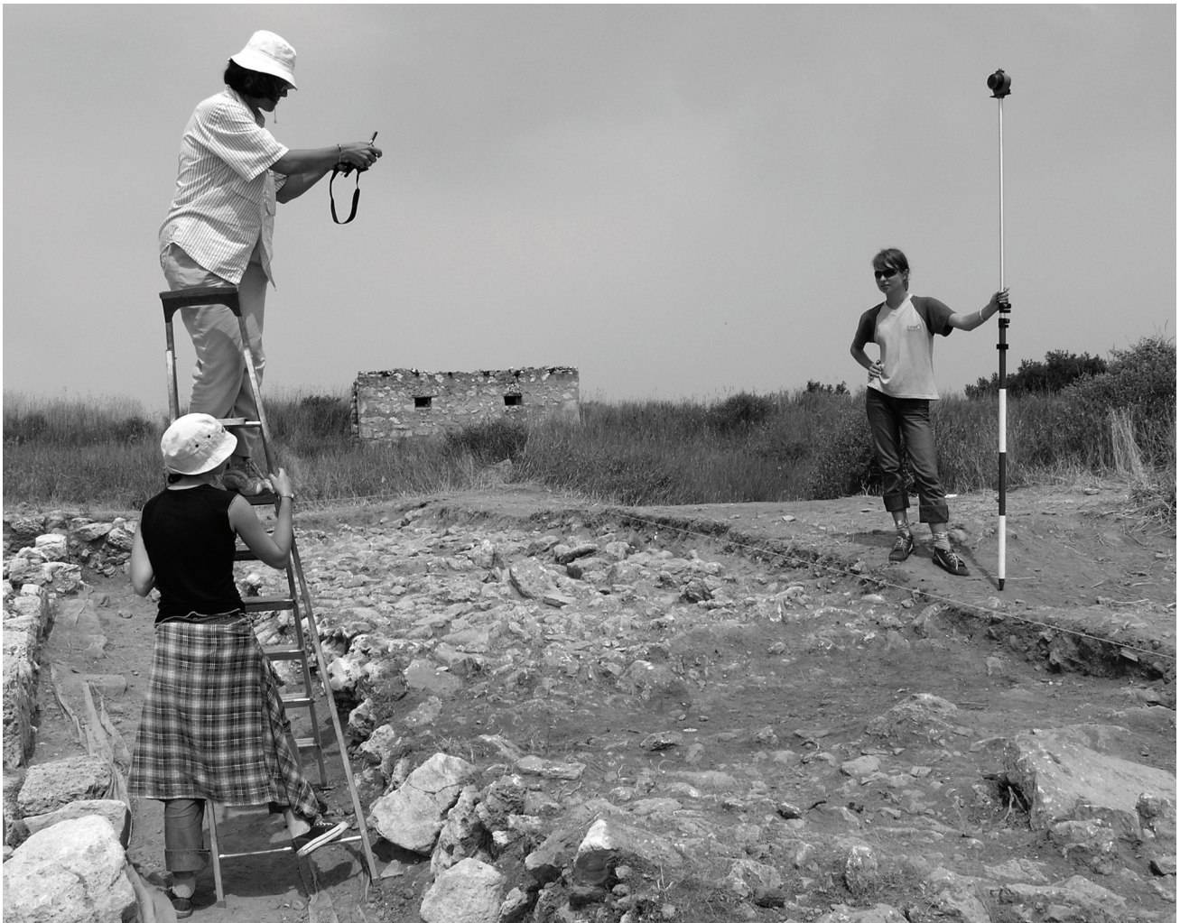
Figure 9. Gordana Karovic uses a roughly-leveled camera to take photographs of the rubble layer covering the stenopos for georeferencing.
