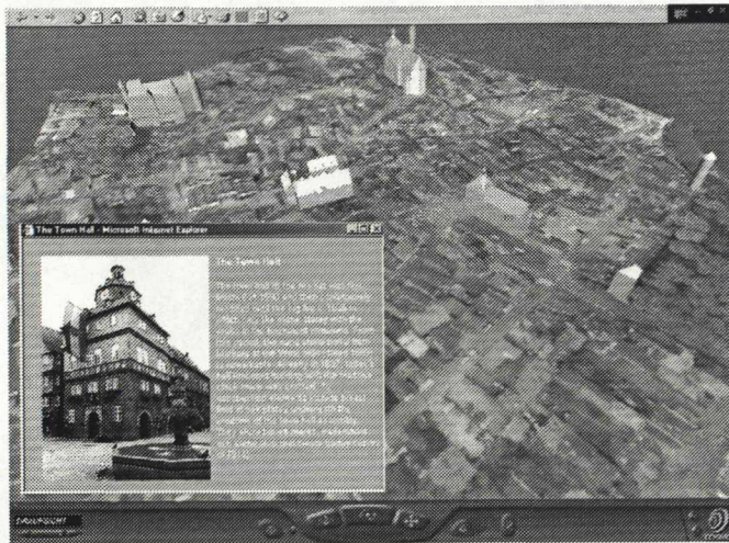
Figure 9: Orthophoto, DTM and buildings of particular interest in a VRML-File with links to detailed description
