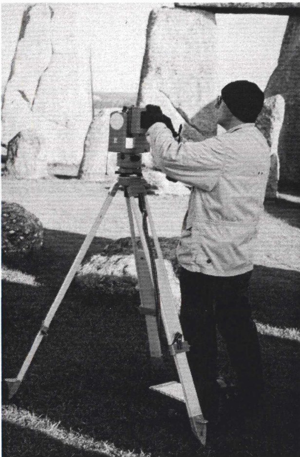
Figure 6.6: Wild P31 metric camera in use at Stonehenge.
