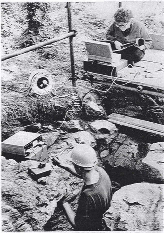
Figure 19.4: The Tracker in use at Torbryan to record reference points on the edge of the fissure. (Photograph : Cath Price).
