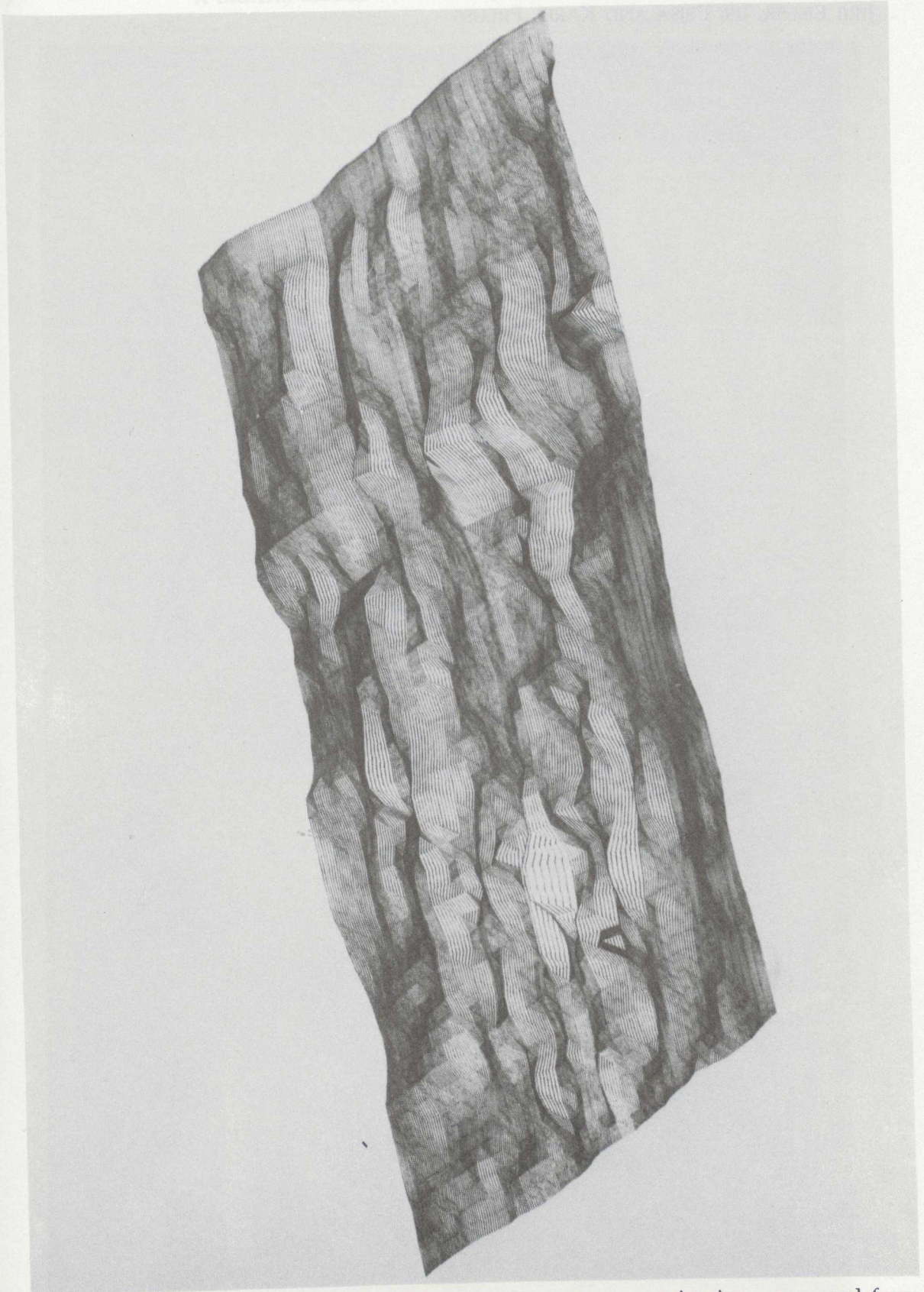
Figure 7.6: The Mortuary Temple of Raneferef—an axonometric view processed from the data of the geophysical survey
