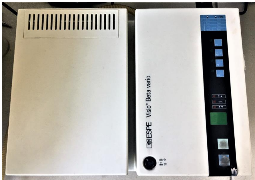
Figure 20: Light curing unit for final curing of veneering composite
