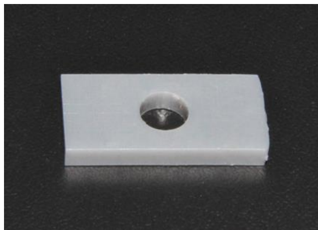
Figure 17: 3D printed bonding jigs
