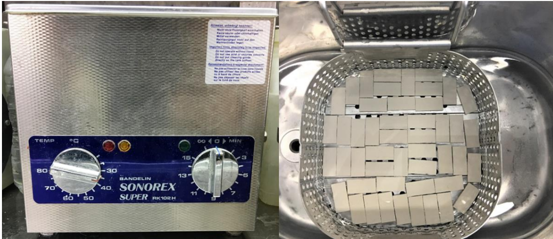
Figure 9: Ultrasonic cleaning of specimens via Sonorex device
