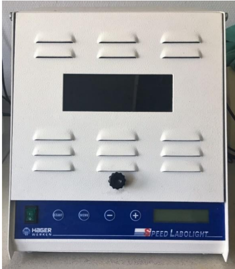
Figure 19: Light curing unit of Visiolink primer
