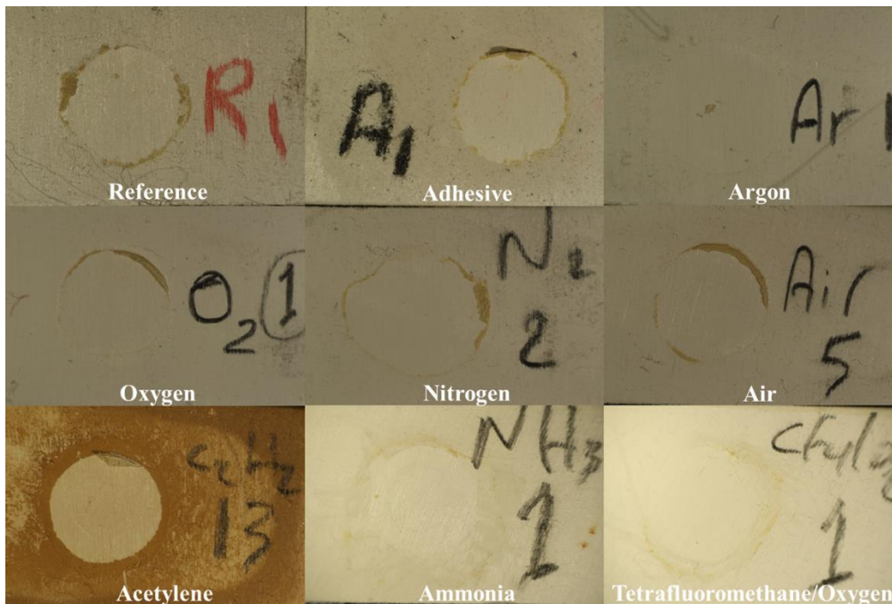
Figure 42: Ceramic filled PEEK specimens showing exemplary adhesive failures after shear bonding strength testing
