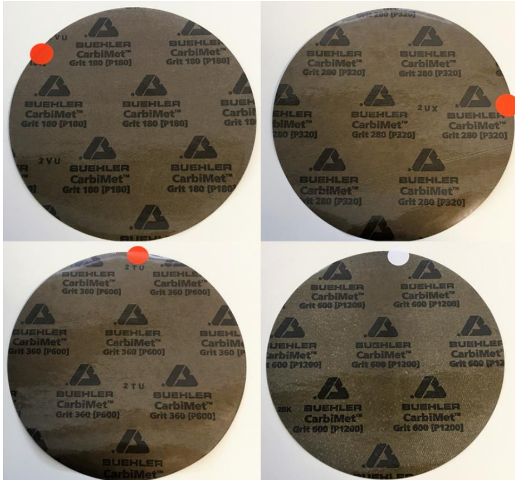
Figure 6: Different types of polishing discs used to standardize the surface roughness of the specimens
