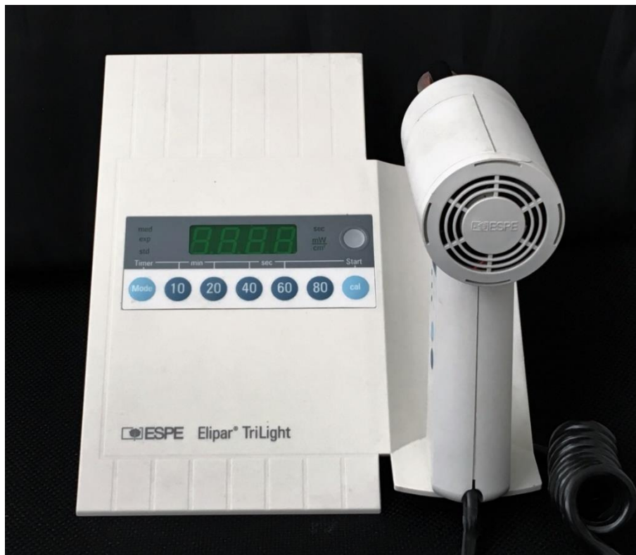
Figure 18: Light curing unit for opaquer and veneering composite
