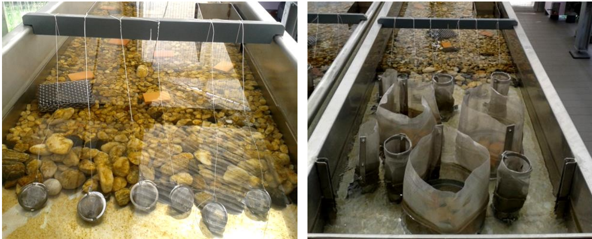
Figure 82: Left: Six enclosures for P. antipodarum fixed with a nylon thread to a beam at the bottom of the respective streams; right: arrangement of three exposure vessels for G. fossarum and six exposure vessels for L. variegatus at the bottom of the respective streams.
