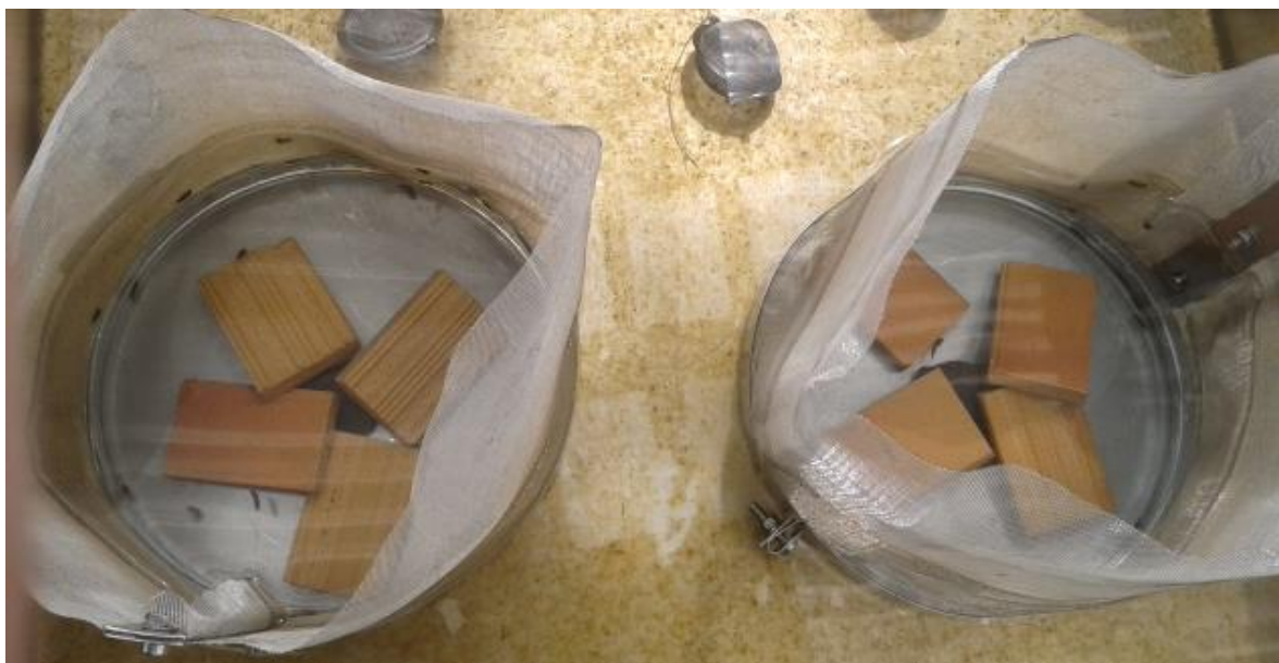
Figure 83: Exposure vessels containing 20 individuals of G. fossarum along with 4 unglazed ceramic tiles, 3 crushed stones and 15 conditioned leaf discs of A. glutinosa
