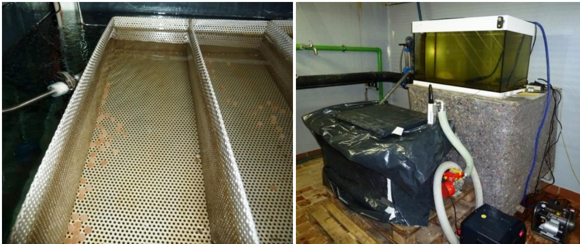
Figure 124: Exposure design of brown trout eggs/larvae directly at the wastewater treatment plant and control station at the Lake of Constance. Eggs were placed in metal sieves (left) within a flow-through system. At the wastewater treatment plant, a second aquarium connected the effluent and exposure aquarium to adjust the temperature and oxygen content (right).
