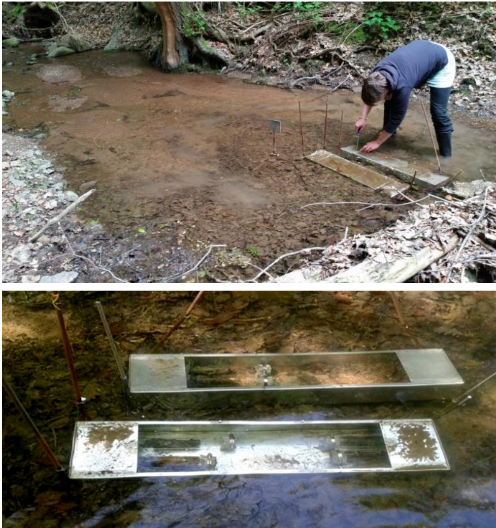
Figure 133: Top: Stainless steel boxes closed with metal grids; bottom: stainless steel boxes in the stream containing 5 and 6 glass tubes respectively as a control set-up, glass tubes including 20 individuals of G. fossarum and 10 conditioned leaves of A. glutinosa .
