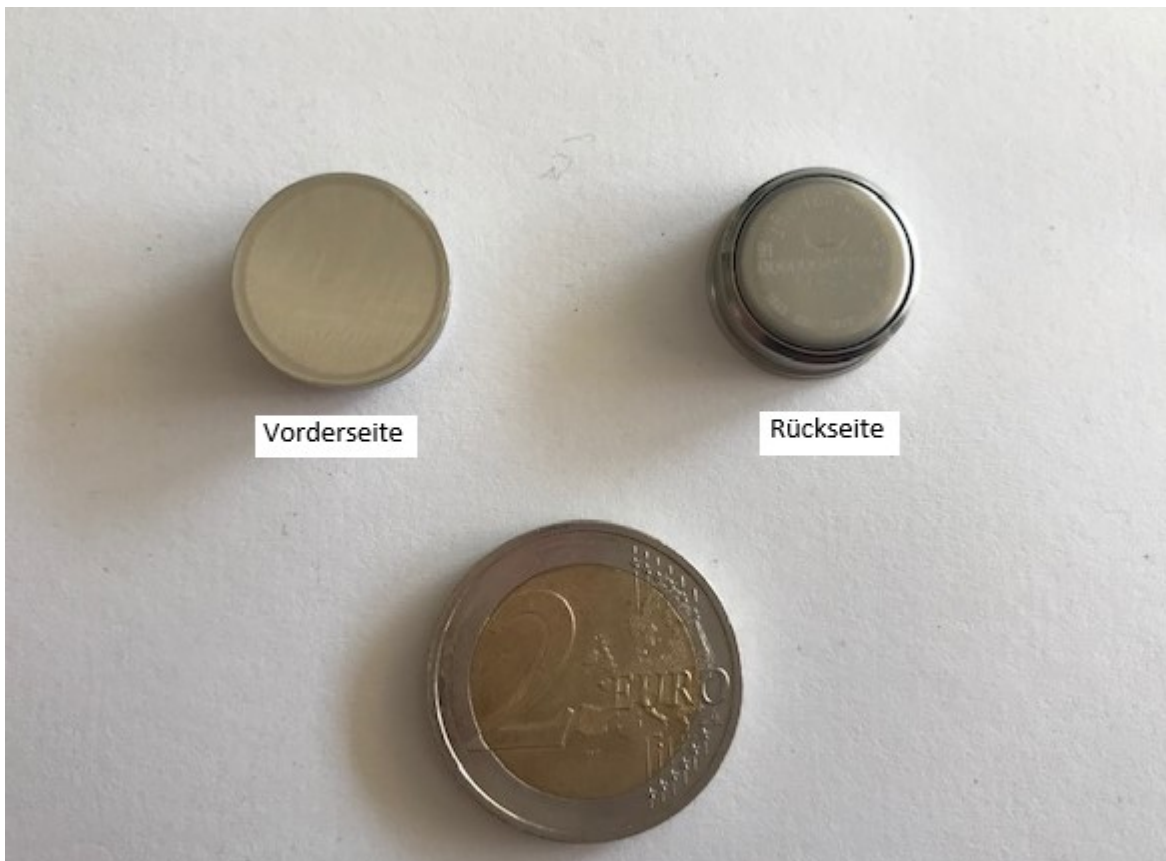
Picture 1: Front and back of an iButton (DS1922L)
