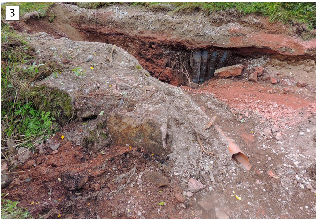
Figure L: Rappenloch. Details 1 shows extraction point for samples RP. 131.6, while detail 2 shows the level of overgrowth as well as extraction point for RP.126.1. These spots were previously dug out by local rock hunters. Detail 3 shows sample collection points for RP.132.7 and RP.134.9, with an exposed clay matrix with overlying sand due to construction activities.
